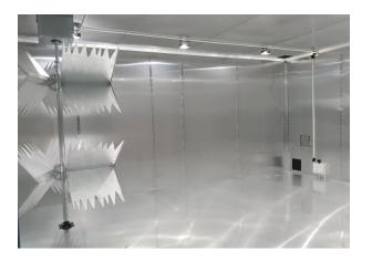
Reverberation chambers are specialized EMC testing facilities for conducting immunity tests on electrical and electronic devices. While most common semi-anechoic chambers have absorbent walls and ceilings with conductive floors, reverb chambers are completely covered by highly conductive walls, ceilings and floors and have metal stirrers, which radiate over the whole device under test.
